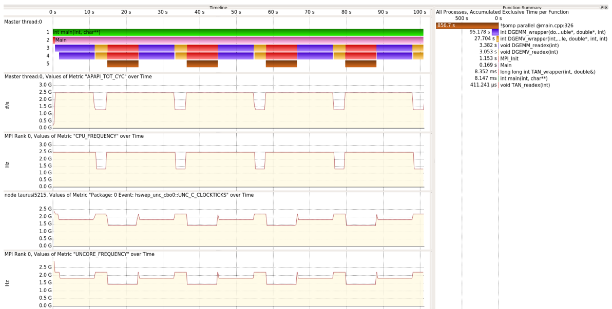
Figure 3: Vampir trace showing the APAPI.TOT_CYC and UNC_C_CLOCKTICKS recorded using the Score-P APAPI and uncore plugin respectively
