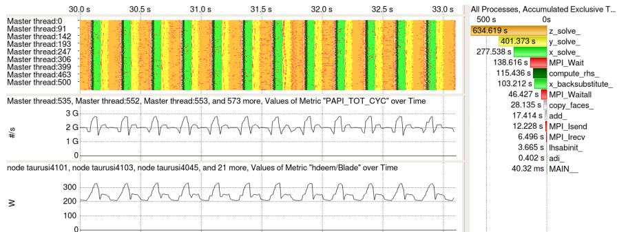
Fig. 9: MPI parallel NPB BT (576 ranks). Left side (from top to bottom): Executed functions (function names on right panel), average frequency of involved processor cores, average power consumption of nodes.
