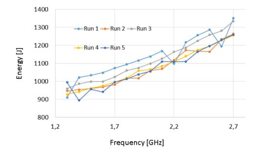
Energy consumption of the SeisSol application at different compute nodes.
