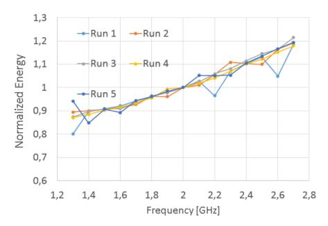
Normalized energy consumption of the SeisSol application at different compute
